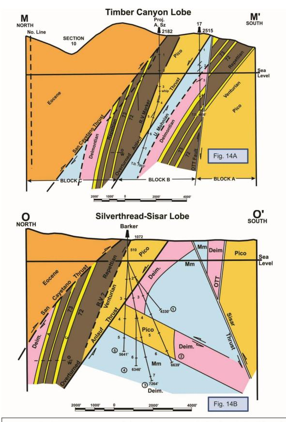
Figure 14. R.L. Hester cross sections of the Timber Canyon and Silverthread-Sisar lobes of the San Cayetano thrust fault (1977). See text for Hester's descriptions of the thrust fault, complex subthrust structural geometry and evolution, and oil traps.
