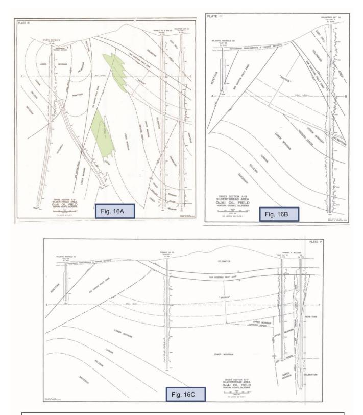
Figures 16A-C. Cross sections of the Silverthread area, Ojai oil field (Mitchell, 1968). Sections show the complex nature of the oil field in the footwall block of the San Cayetano thrust fault. Note up-dip and lateral trapping provided by the Big Canyon fault. Only Figure 16A shows the oil zones and are from DOGGR (1992).
