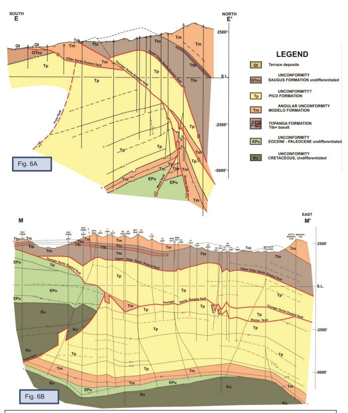
Figure 6A. Dip cross section E-E' of the Aliso Canyon oil field (modified from Lant, 1977). Figure 6B. Strike cross section M-M' (modified from Lant, 1977). Note the thick Pico Formation section in the footwall of the Santa Susana fault, and the thick Topanga and Monterey Formations section in the hanging wall of the Santa Susana fault. Lant's sections also show that the Santa Susana fault consists of two strands with the younger strand offsetting and folding the older and higher strand.
